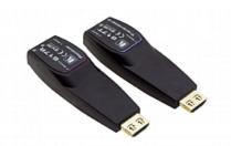
617R/T is a compact fiber optic transmitter and receiver capable of extending HDMI signals over fiber optic cable. This set of extenders supports 4K@60 (4:4:4) resolution up to 656 feet (200 meters) on a dual LC multi-mode fiber cable
